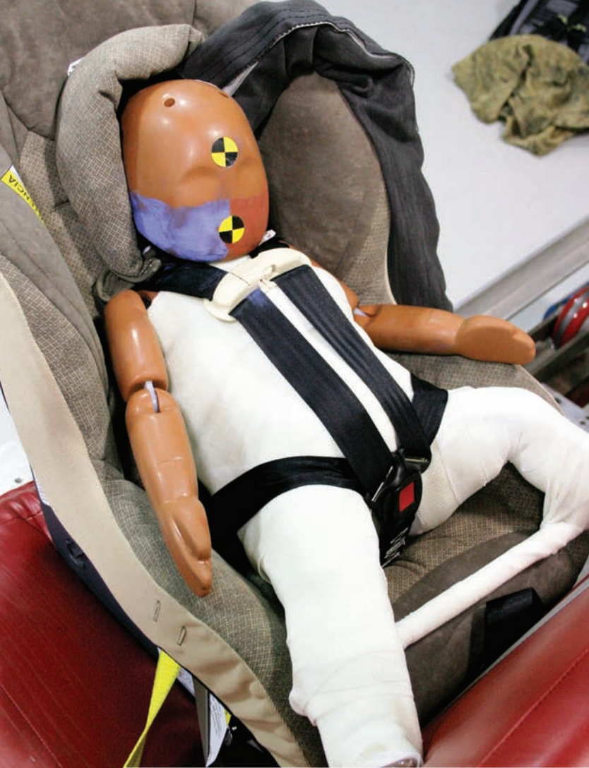
Ready to ride, the crash test dummy representing a nine-month-old, is casted and secured in the car seat. The blue chalk on the face is to determine head movement during the crash event.
