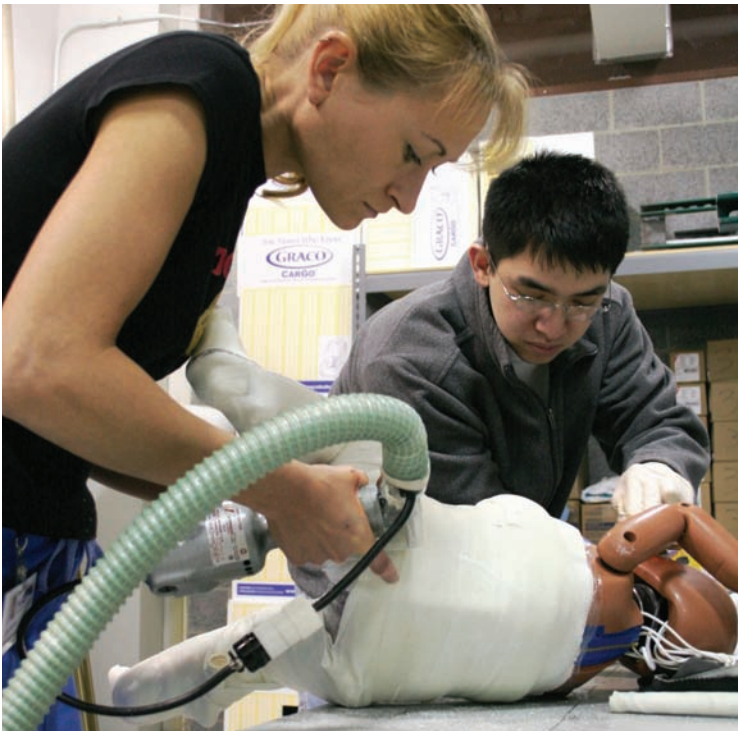
Dr. Julie Zielinski, orthopedic surgery resident at McLaren Regional Medical Center, cuts the cast off a crash test dummy after a side impact crash test while Kettering student Kevin Xie, a junior from Sterling Heights, wipes off the blue chalk.
